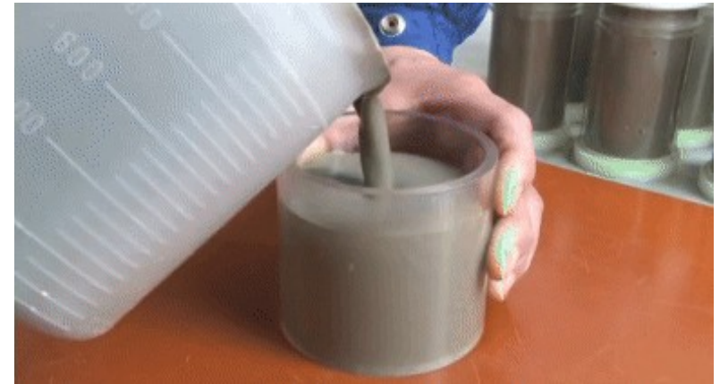
Liquefied Treated Soil
