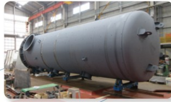
Plate working for plant equipment (Contract-Based Manufacturing Business)
