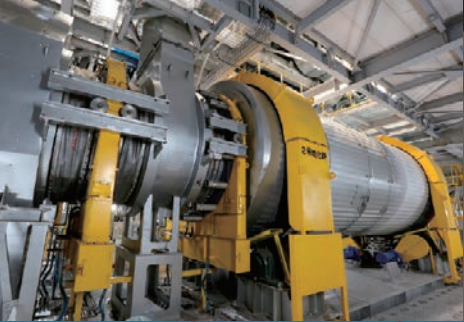
Carbonization furnace constructed by Kawasaki Heavy Industries, Ltd., operating in the facility for manufacturing carbonized fuel from municipal waste in Saikai City, Nagasaki Prefecture (materials provided by Kawasaki Heavy Industries, Ltd.)
