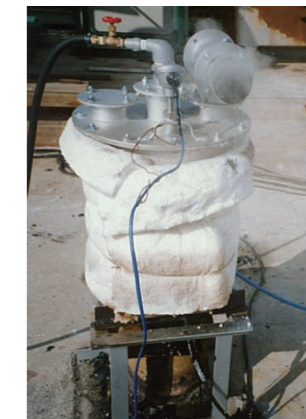
Photo 2: VOCs (odor-causing components) generation apparatus
