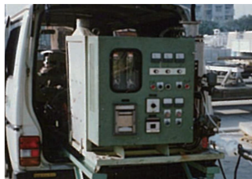
Photo 7: Continuous total hydrocarbon analyzer (FID)
