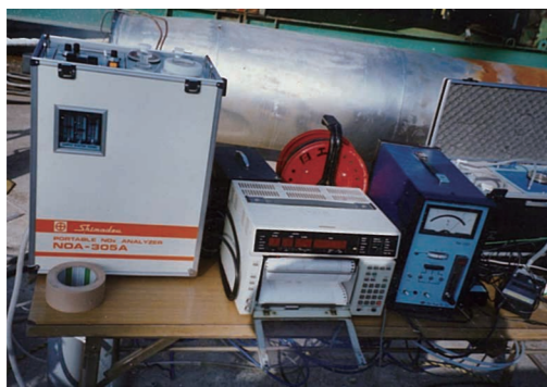
Photo 6: From left: NO x concentration analyzer, recorder, oxygen concentration analyzer, and other instruments
