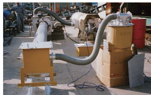
Photo 1: Overall view of the VOC deodorization experimental apparatus
